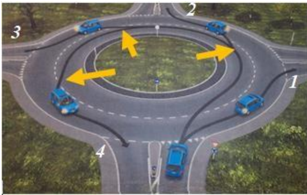
Roundabout intersection with one entry-exit lane and two lanes in the circle
