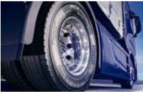
Tireless pneumatics are now in use so-called "Tubeless".
